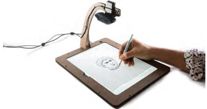
Figure 6. Livedraw 2015; System consists of a thin USB-powered LED lightbox, encased in a custom fabricated casing made of Masonite that includes an appendage for holding the camera in the ideal location, and a USB HD Webcam
