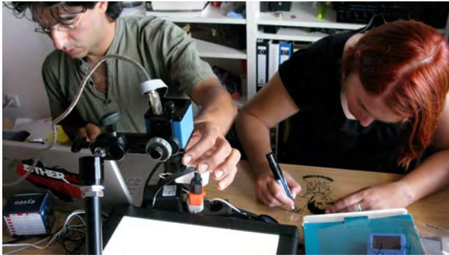
Figure 4. Livedraw Hardware v1: Momeni (left) and Schmid (right) collaborating on a livedrawing performance; System consists of a light box, digital camera with C-Mount lens and custom software. Schmid draws with pens/markers on transparency paper; digital camera captures image for manipulation in software
