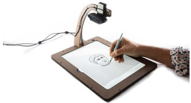
Figure 6. Livedraw 2015; System consists of a thin USB-powered LED lightbox, encased in a custom fabricated casing made of Masonite that includes an appendage for holding the camera in the ideal location, and a USB HD Webcam
